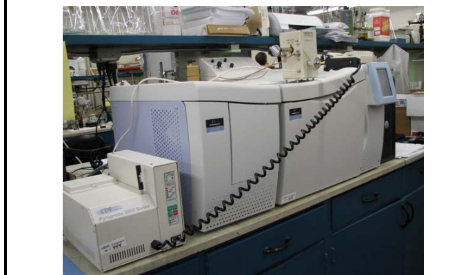
Figure 2: Running Sample in Pyrolysis-GC/MSFID
