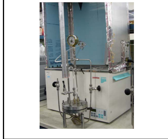
Figure 9: Ready to Start Permeability Test
