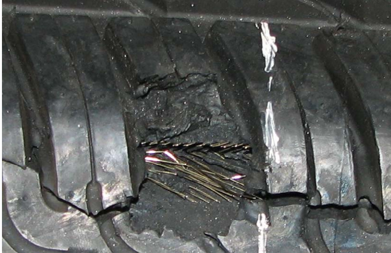
Figure 9. Photograph of Tire Section After Failure: Tire with IPR = 1.45 (100-phr bromobutyl rubber) failed at 55.8 hours (top picture); Tire with IPR = 2.0 (80/20 BIIR/NR) failed at 49.0 hours (middle); and Tire with IPR = 2.65 (60/40 BIIR/NR) failed at 39.7 hours (bottom).
